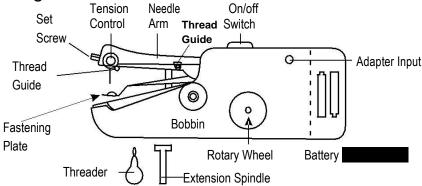
Notes: always use rotary wheel to move needle. Never press or pull directly on needle arm to avoid damages to internal mechanism
