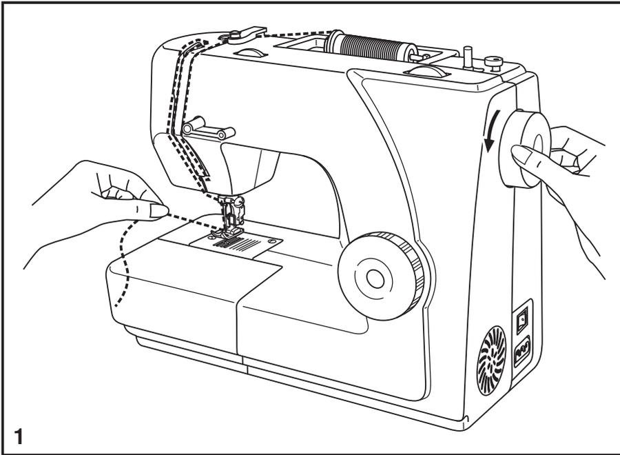
Gently pull on the upper thread to bring the bobbin thread up through the needle plate hole (2).
