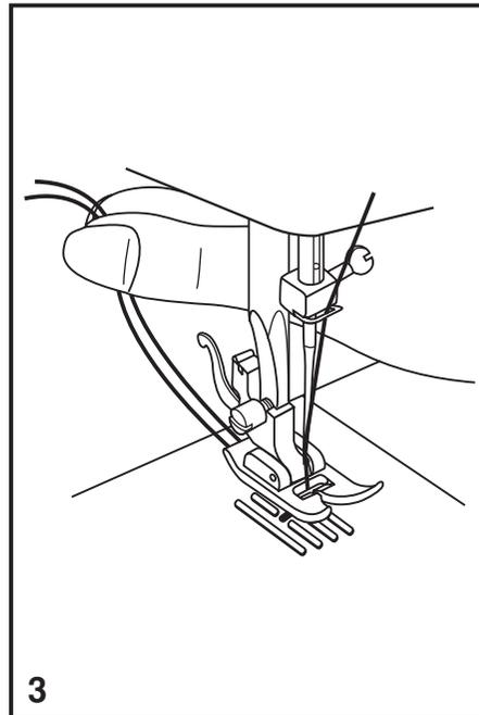
Lay both threads to the back under the presser foot. (3)
