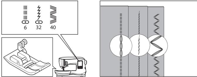
We recommend that you use a needle for knit and synthetic fabrics to prevent skipping stitches and thread breakages. See page 9 for needle recommendations.
