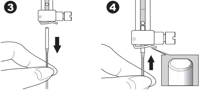
5. Tighten the needle clamp screw.
