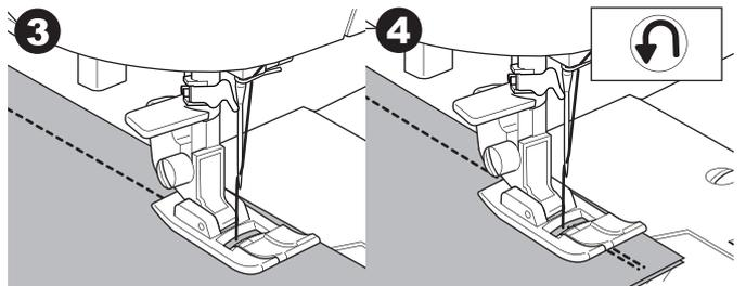
5. Release Reverse button and sew until end of seam.
