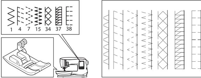
Place fabric so that the needle falls near the edge of the fabric when using the All-Purpose Foot.
