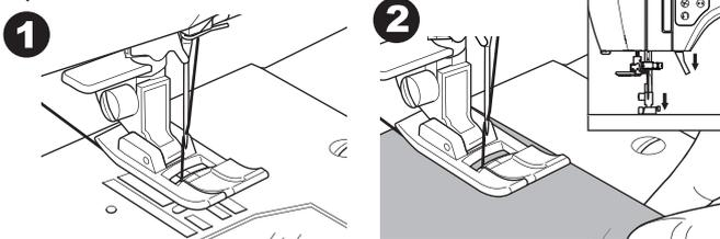
3. Hold back upper thread and press the Start/Stop button or press the foot controller pedal. Keep holding thread after sewing a few stitches. Lightly guide the fabric while sewing. You can regulate the sewing speed by pressing the Speed Control buttons or the foot control. The buttons are used to set the speed when using start/stop button and also sets the top speed when using foot control.
