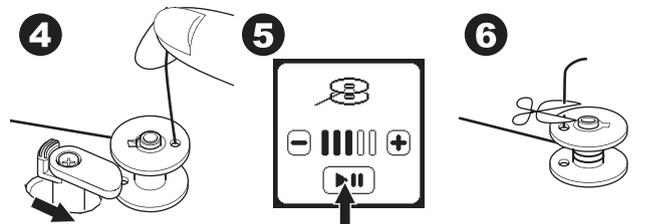
7. Start the machine again by pressing the Start/Stop button on screen. You can adjust winding speed by pressing "+" (faster) or "-" (slower) button on the screen.
