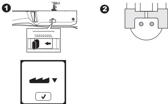
3. Adjust the stitch width so that the needle enters the left hole of button.
