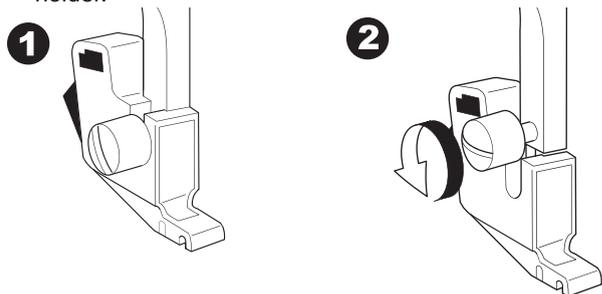
3. To replace the holder, pull up the holder as far as it will go from bottom of presser bar.
