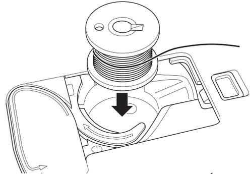
2. Draw thread into notch (a) while holding the bobbin lightly with your finger.
