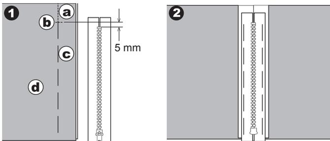
3. Attach the Zipper Foot. Attach the left side of the presser foot pin to the presser foot holder when sewing the right side of the zipper, and right side of the presser foot pin to the holder when sewing the left side of the zipper.
