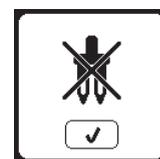
This message will appear when stitch width is adjusted to the limit. Press the the “✓” button to continue.
