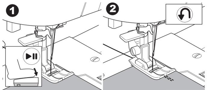
3. Release the Reverse button and sew forward until reach the end of seam.
