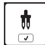
This message will appear when a stitch that cannot be used with twin needle, is selected. Press the the “✓” button and select another pattern or reset the twin needle program.
