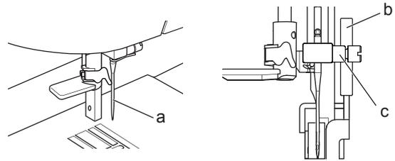
3. Slide the attaching head from your left to right so that it is fitted into the presser bar. For easier access, lower the needle slightly by turning the hand wheel toward you.
