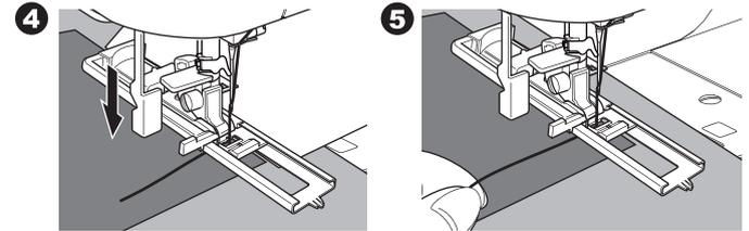
6. Machine will sew bar-tack or darning stitch, as shown. Machine will stop automatically when the pattern is finished.
