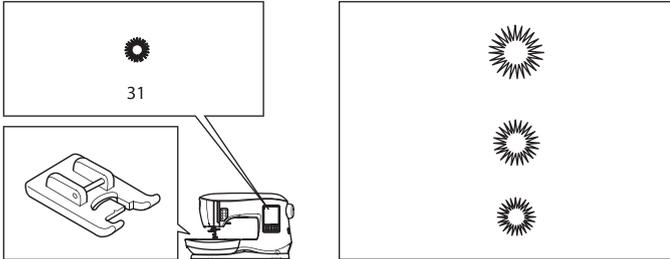
1. Place the fabric under the presser foot and lower the presser foot. Start the machine.
