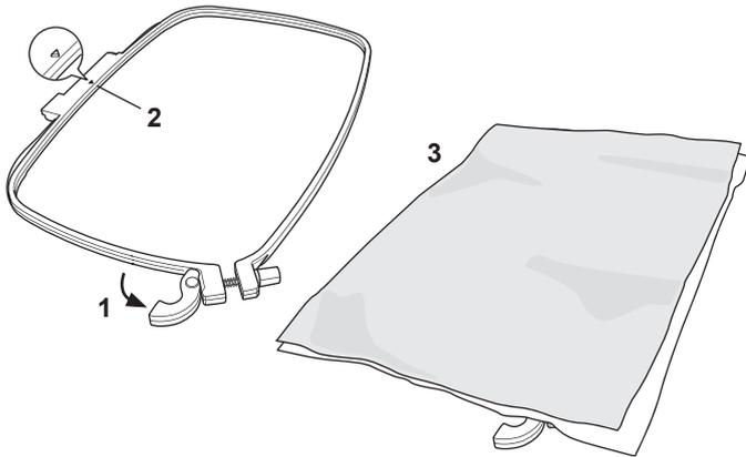
4. Place the inner hoop on top of the fabric with the small arrow at the left edge and push firmly into the outer hoop.
