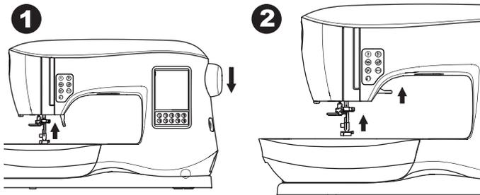
3. Remove the presser foot by pushing the presser foot release lever toward you.
