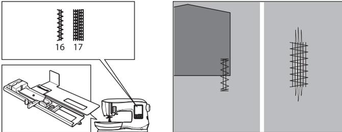
1. Adjust slide on base of Buttonhole Foot according to the length of the bar-tack or darning to be sewn.
