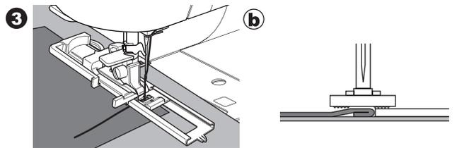
4. Lower the Buttonhole Lever completely.
