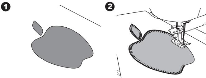
When sewing sharp angles or curves, bring the needle to its lowest position and raise the presser foot. Use needle as pivot and turn fabric.
