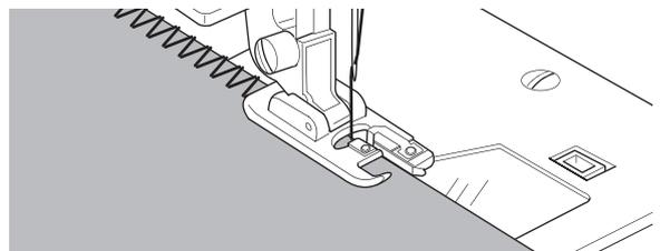
No. 3, 33, 35, 36 are designed to sew the seam and seam finish at the same time.
