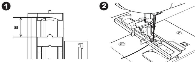
3. Position fabric under presser foot so that the starting point is on the thick area.
