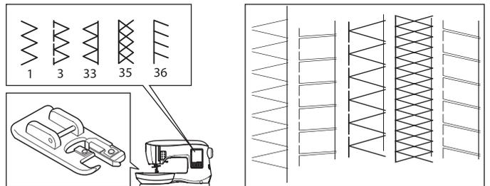
Line up the fabric against the guide plate of the overcasting foot so that the needle falls near the edge of the fabric.
