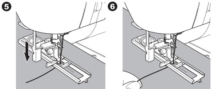
7. Machine will sew the buttonhole in the order as shown and stop automatically after sewing.
