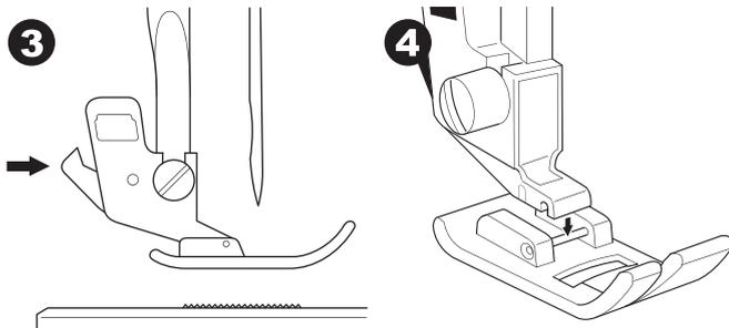
5. Lower the presser foot lifting lever and the presser foot will snap into place.
