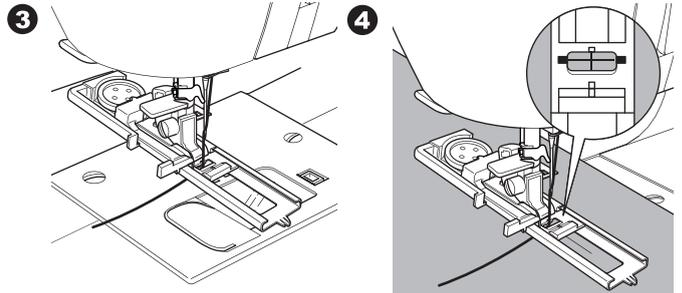
5. Lower the Buttonhole Lever completely.
