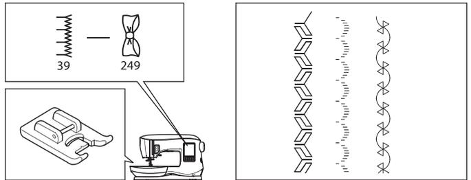
To customize the continuous decorative stitch pattern, you may adjust the length and width of pattern. Experiment with fabric scraps until you achieve the desired length and width.
