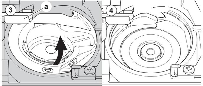
5. Replace the bobbin holder into the hook race so that the tip (b) fits to the stopper (c) as shown.
