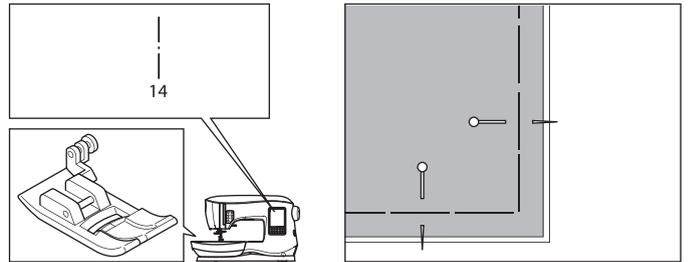
1. Place the fabric under the presser foot and then lower the presser foot lifter.
