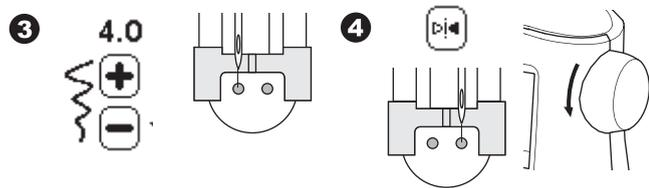
5. Set the number of stitches to sew on the button by pressing the + and - buttons. Eight stitches is standard.
