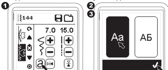
4. Press the desired letter directly. Press the Character tabs (located at the bottom of the LCD screen) to change lower case, numbers, etc.
