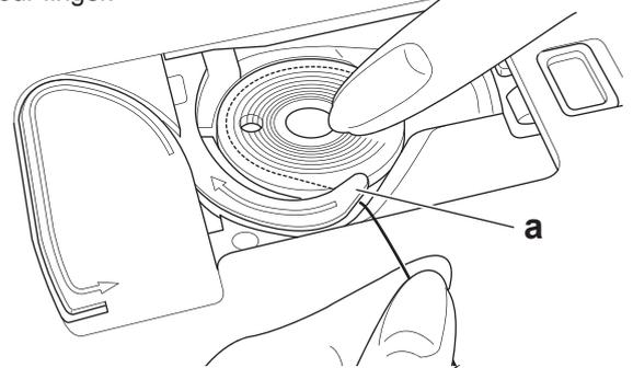
3. Pull thread along the groove, up and around the top, to the left, then down. Pull thread to the right to cut the thread.
