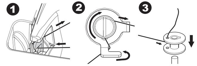
4. Hold the end of the thread and push bobbin stopper to the right. When the bobbin winding screen appears, press the Start/Stop button on the screen to start winding.
