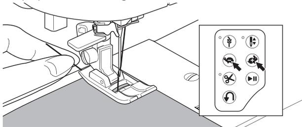
4. When you reach end of seam, press the Start/Stop button to stop sewing or release the foot controller pedal.
