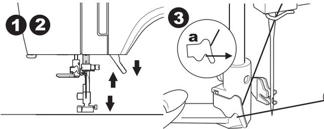
4. Push the lever as far as it will go. The threader will turn and the hook pin will go through the needle eye.
