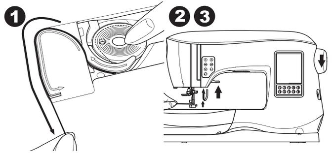
4. Pull upper thread lightly. Bobbin thread will come up in a loop.
